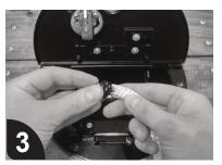
Screw the new line into the rope attachment.
