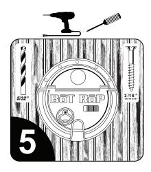
With the **Bot Rop** in place, use a 5/32 inch drill bit to pre-drill the 11 holes located around the top of the unit. Then secure the unit to the dock with the provided screws. Keep in mind that 6 holes are concealed under the lid.
