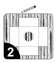
Lay the template on dock with the outer edge of the hole 3 inches from the edge of the dock. Avoid placing template over joist below the dock. Trace the circle opening with a pencil on the location where you will install the Bot Rop
