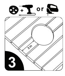
Remove the template and use the Power Drill with the Hole Saw Bit or the Jig Saw to cut on the pencil line to create the opening in the dock. Make sure the hole is 3 inches from the edge of the dock.
