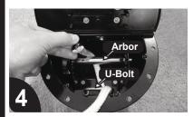
Tether the line back underneath the u bolt, then the arbor and screw the new rope into the arbor.
