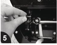
Unscrew the set screw to release the rope back into the canister.
