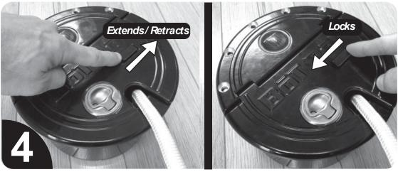
With the rope attached securely to the boat, you can push the *Tidal Adjustment Switch* to the right. This allows the rope to extend and retract freely in rough or tidal conditions. If you push the switch to the left, it locks the rope into place.
