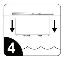
Place the **Bot Rop** in the opening in the dock with the logo side up allowing the majority of the unit to be suspended below the dock.
