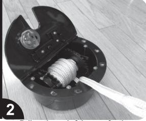
Pull on the end of the rope for the desired length necessary to reach your boat.
