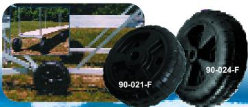
Wheels are available in 18" or 24" diameters and up to 700 lb. capacity per wheel. These tough, rigid wheels offer stress, crack and impact resistance. They roll easily over virtually any terrain and will not rust on the axle. Use for roll-in docks or boat lifts. All wheels accept a 17/8" O.D. axle. HD Wheel capacity exceeds 700lb ea.
