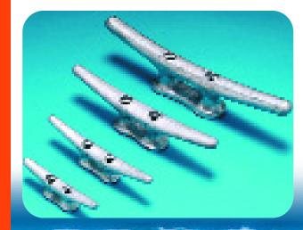
These are your traditional, Cast Iron, Hot Dipped Galvanized Dock Cleats. The mounting holes are recessed with a hexagonal shape to stop the head of a carriage bolt from turning while securing the cleat to a surface. This eliminates the need for two wrenches when securing, or in some cases an extra pair of hands.
